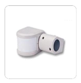
A-ES5 series is a passive infrared SenSwitch with two dual element sensor built-in to provide 200° ultra wide angle detection. It can automatically switch on the indoor or outdoor lighting by sensing the presence of human body.
